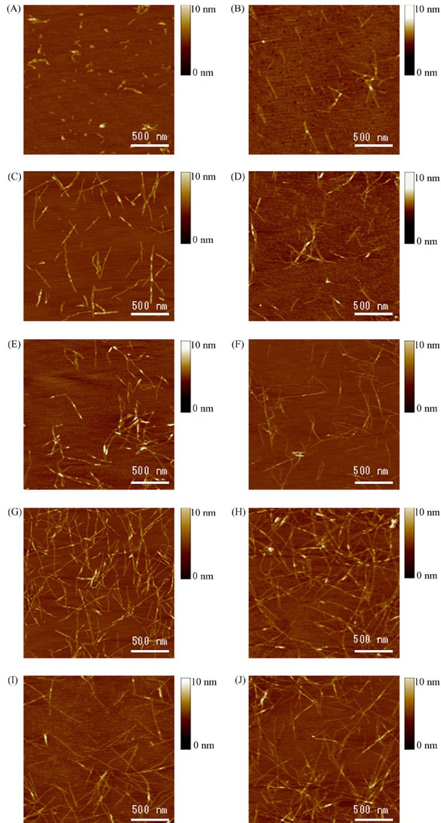
**Figure 4** AFM images of RADA16-I nanofiber at various time points after sonication. The observations were made using AFM immediately after sample preparation. (A) 1 min after sonication; (B) 2 min; (C) 4 min; (D) 8 min; (E) 16 min; (F) 32 min; (G) 64 min; (H) 2 h; (I) 4 h; (J) 24 h. Note the elongation and reassembly of the peptide nanofibers over time. By  $\sim 1$ –2 h, these self-assembling peptide nanofibers have nearly fully re-assembled.
