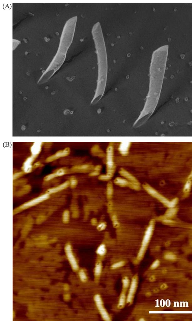
**Figure 11** (A and B) TEM and AFM image of designer lipid-like peptide surfactant. These peptides undergo self-assembly to form nanotube structure. Quick-freeze/deep-etch TEM image of Ac-V<sub>6</sub>D-OH dissolved in water (4.3 mM at pH 7). The TEM images show the dimensions, ~30–50 nm in diameters with openings of nanotube ends. Note opening ends of the peptide nanotube may be cut vertically. The strong contrast shadow of the platinum coat also suggests the hollow tubular structure.
